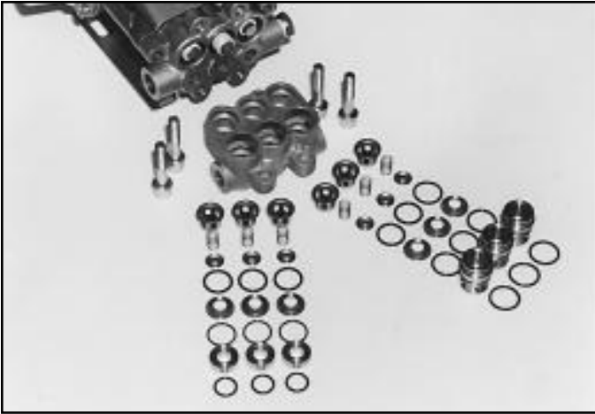
Discharge and Inlet Valve Assemblies
